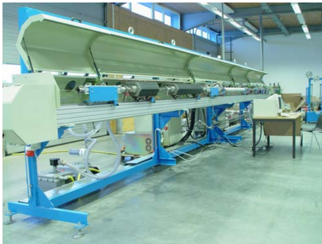
Figure 3: Plasma wire heat and surface treatment machine for high-speed applications with 2 electrodes, flexible sealing system and combined (gas and water) cooling system.
